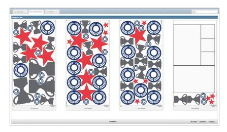
usage, and providing faster file-handling and greater printer throughput. It even has features to handle the unavoidable remnant area of nested jobs. You can reduce scrap by having leftover media cut and turned into "standard sheet sizes" for later use, or simply hold jobs on the last layout for later printing.
