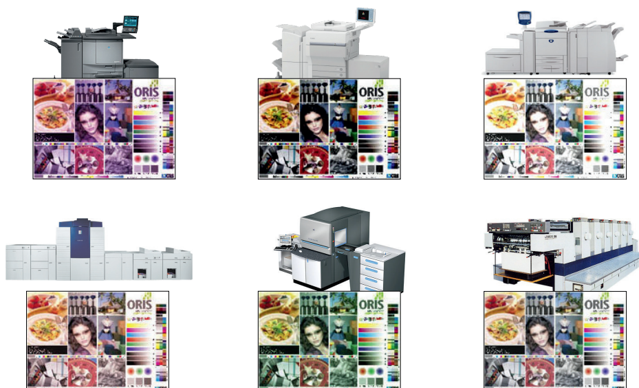
Fig. 2.17: Simulation of the resulting colour appearance, when offset data is used for output „1:1“, i.e. based on four 1-dimensional curves (“Device Mode Transform”) on different digital printing systems. Source: CGS
