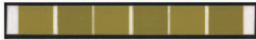
Under lightning with a color temperature of 5000k, the color temperature indicator shows no stripes.
