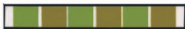
Under lighting with a color temperature above or below 5000k, the color temperature indicator shows stripes of different shades of green and olive.
