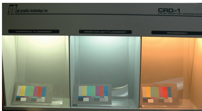
Fig. 2.2: Identical hardcopy prints under three different light sources (left: office illumination – „Cool white Fluorescent“, middle: daylight simulator D50 according ISO 3664, right: tungsten source)..
