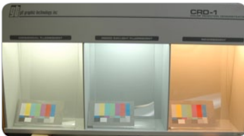
Figure 37: Identical test prints under three different light sources (left: commercial fluorescent, middle: D50 Simulator, right: incandescent)
